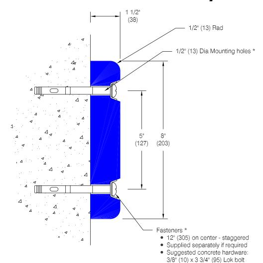
\* Standard bumper is supplied undrilled and with no mounting hardware. Hole spacing shown for bumpers 48" (1219) and longer. Contact factory for hole spacing on lengths shorter than 48" (1219).
